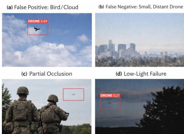
Fig. 4: False Positives and False Negatives in drone detection
